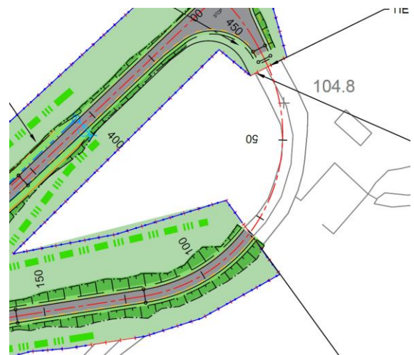
Figure 2-9 Tie in between existing and new road alignment
