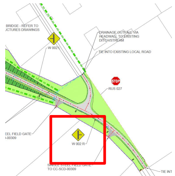
Figure 2-10 Location of Warning Sign
